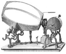
**Before Edison.** French "phonautograph" from the 1850s (*above*) traced sound waves onto paper (*right*) for sight-reading, not playback.
